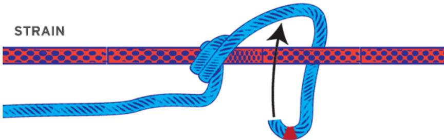
2. Then the bitter end doubles back to a hitch taken on the side of the turns away from the strain.
