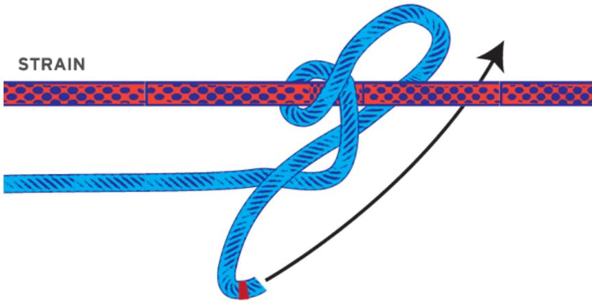
1. Two turns are taken around the line in the direction of the tension, the second inside the first.
