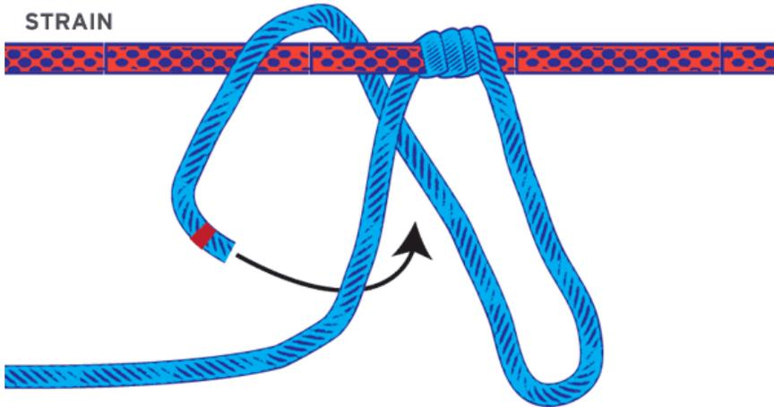
1. Three turns are taken away from the direction of the strain, then the bitter end crosses under the turns and over the line under tension.
