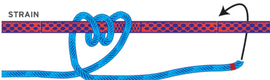
1. Three turns are taken in the direction of the strain.
