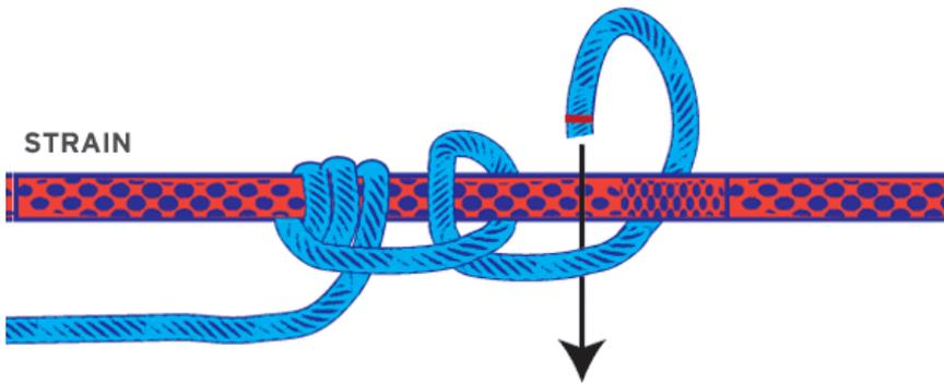
2. Then two half-hitches are used to finish it off.
