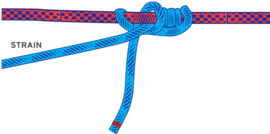
3. Take the bitter end over the top of the line under tension and through the loop. Pull tight.
