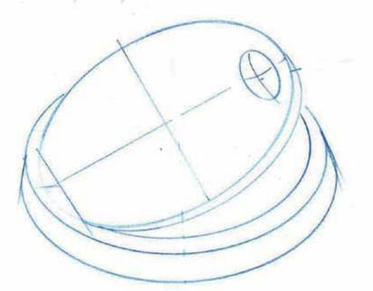
LID D - Push down lever to open lid Leverage mechanism. Push down on lever to open lid. Could be tied in with spring release method.
