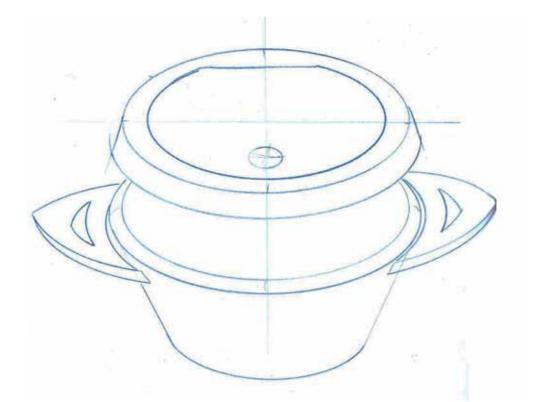
Spring loaded lid - inspired by bin lid mechanism. Push down to open - lid operates on hinge. Easy to close quickly.
