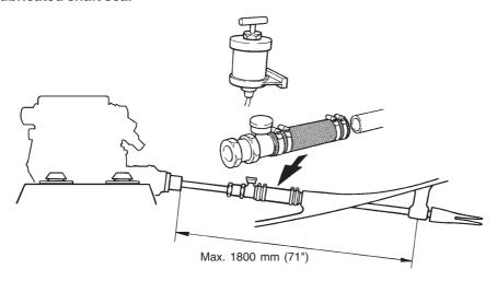
When using a flexible shaft seal and flexible engine suspension, a flexible shaft coupling must **not** be fitted.
