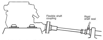
When using a rigid shaft seal and flexible engine suspension, a flexible shaft coupling must be fitted.
