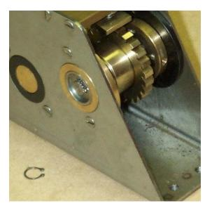
LOOKING DOWN ON 9 TOOTH GEAR CRESCENT SHAPED CUT OUT. THIS IS WHERE LEG ON END CAP FITS. THE CRESCENT EFFEC-TIVELY LIMITS THE LOCK/RELEASE MECHANISM. AS THE WASHERS WEAR THE LEG WILL REACH THE END OF THE CRESCENT BEFORE IT LOCKS. SO WITH THE RATCHET NOW LOCKED ALIGN THE END CAP WITH THE LEG IN THE CUT-OUT AS FAR AS IT WILL GO IN THE ANTI-CLOCKWISE DIRECTION, THEN ROTATE 1 TOOTH CLOCKWISE-AND RE-FIT.
