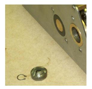
THIS IS THE IMPORTANT PART. HOLDING RATCHET WHEEL TURN THE 9 TOOTH GEAR CLOCKWISE TO TIGHTEN BRAKE MECHANISM. ONCE FINGER TIGHT IT SHOULD BE HOLDING THE RATCHET GEAR FIRMLY, PREVENTING ANY ROTA-TION. (NOTE: WHILE TIGHTENING ENSURE 9 TOOTH GEAR IS OUT OF MESH WITH GEAR ON INTERMEDIATE SHAFT)
