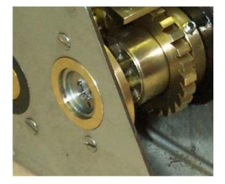
STEP 6 TAP SPLINED SHAFT INTO GEARBOX, LEAVING END CAP IN PLACE
