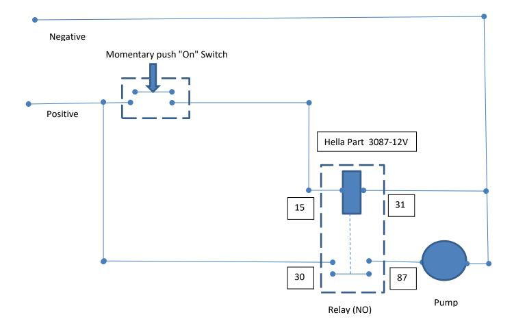
Toilet pump control allows for Momentary push "ON" situated near toilet. Relay uses normally open contacts. This relay can be set to "Delay Off" so water supply pump only runs for predetermined period that has been set on the relay. All voltages for control and actual pump are similar.
