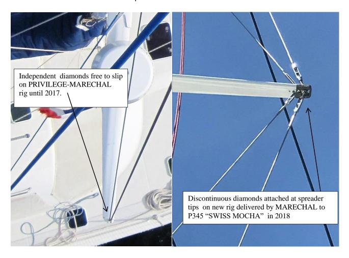
I was personally witness to CATANA breaking 5 masts in a few month in 1999, until they understood the cause to be the independent and slipping double diamonds. The epidemia of dismastings stopped when they attached discontinuous diamonds at spreader tips.
