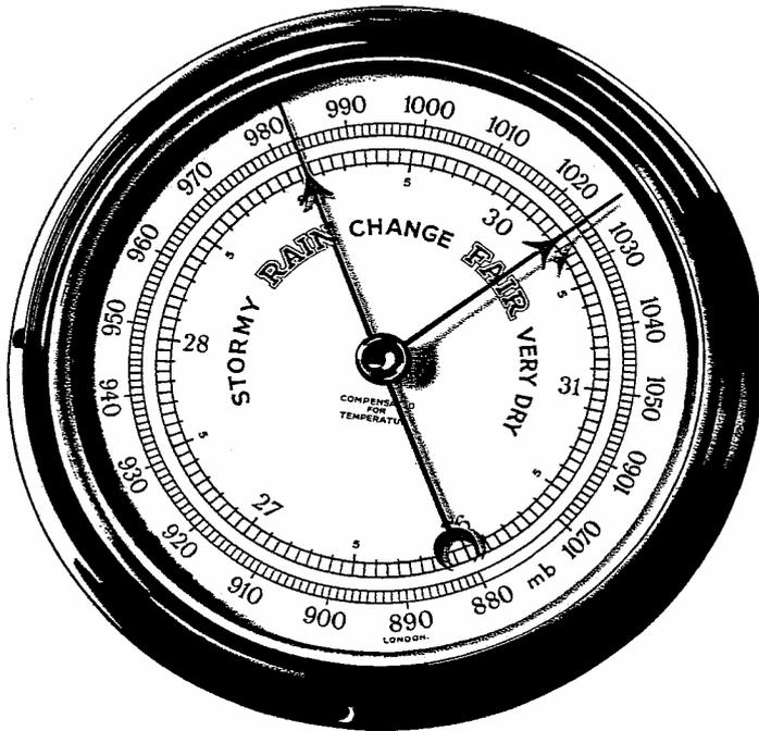
Inside there is a metal cell only partially filled with air. The size of this airtight cell varies with changes in the surrounding air pressure, and these variations are passed on to an indicator needle by a series of levers. It is all mechanical, so no batteries are needed. If the metal chamber cracks then the barometer will no longer work.
