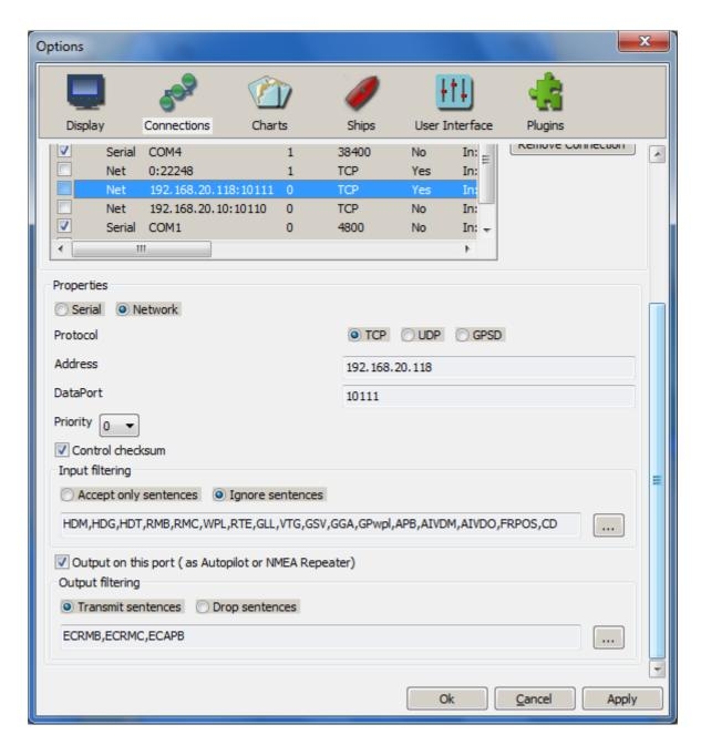
I'm sure theres stuff in there that doesnt need to be, like a lot of the filtering. When I did this I was simply trying to remove everything exraneous, when it worked I left it all alone. Also note that the IP address of the ouput connection is that of the laptop running OCPN, the input connection is to my routers IP address.
