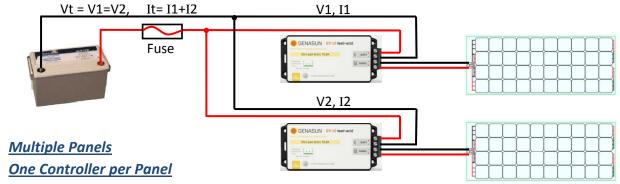
The best solution for multiple panels. Controllers must be able to handle full rated panel voltage and current output. Cables must able to safely handle maximum current, and be sized for 3% volt-drop. Fuse should be max current plus 50%.
