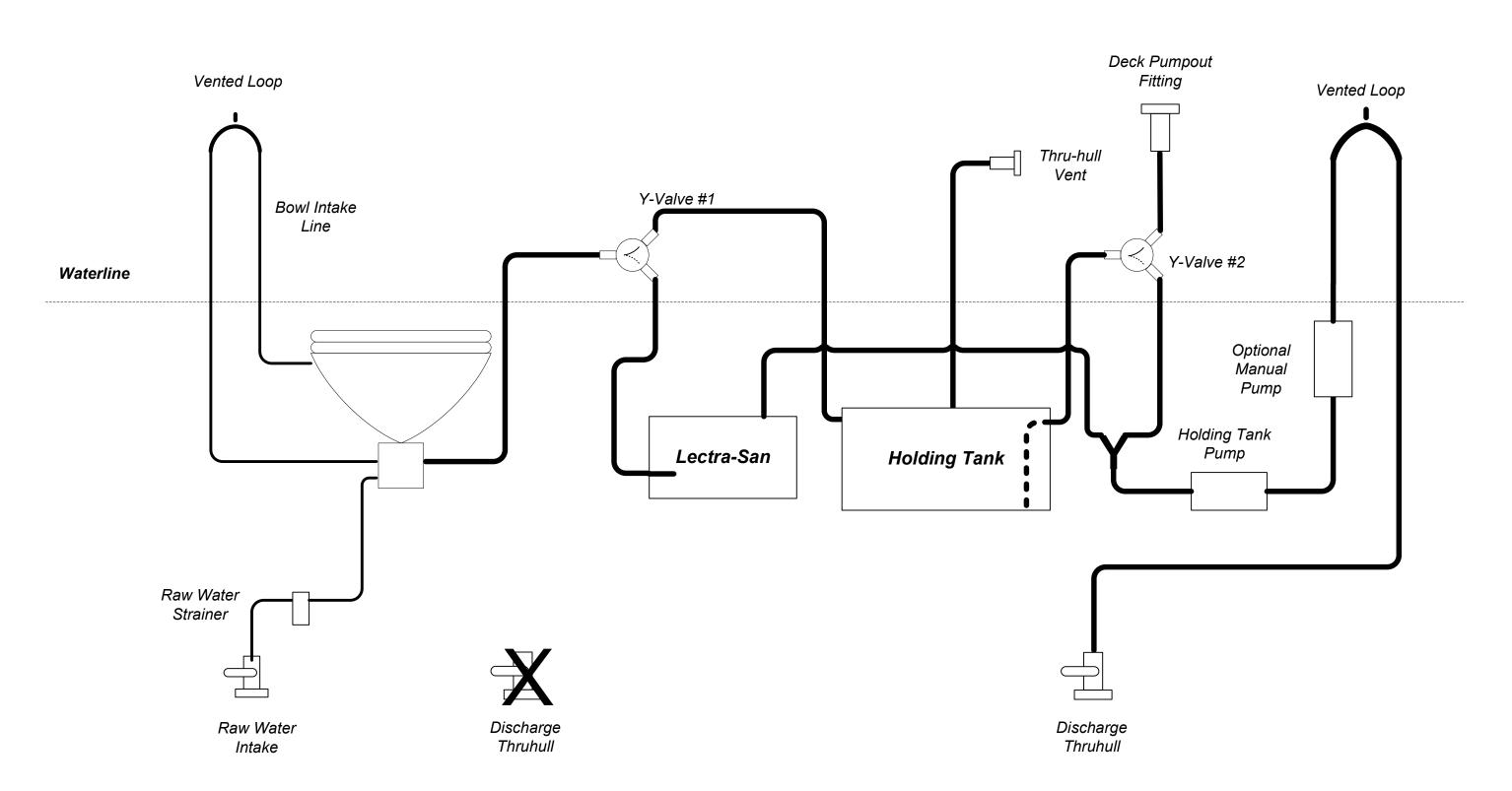
Y-Valve #1 normally set "**Down**" for discharge into Lectra-San Type I MSD. Can be set "**Up**" to fill holding tank when in designated "No-Discharge" areas.
