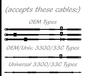
**NOTE:** When properly installed, these engine controls will connect to outboard, stern drive and inboard engines, utilizing Mercury/Mariner<sup>®</sup> and OMC<sup>®</sup> OEM type control cables as well as universal 3300/33C type cables and engine connection kits.
