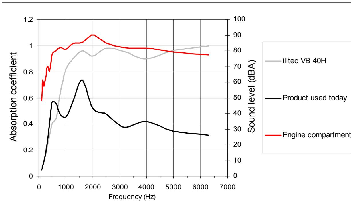
It clearly appears illtec VB40H suits to the problematic. Indeed we have a high absorption where frequencies are the most contributive to the noise level in the engine room.
