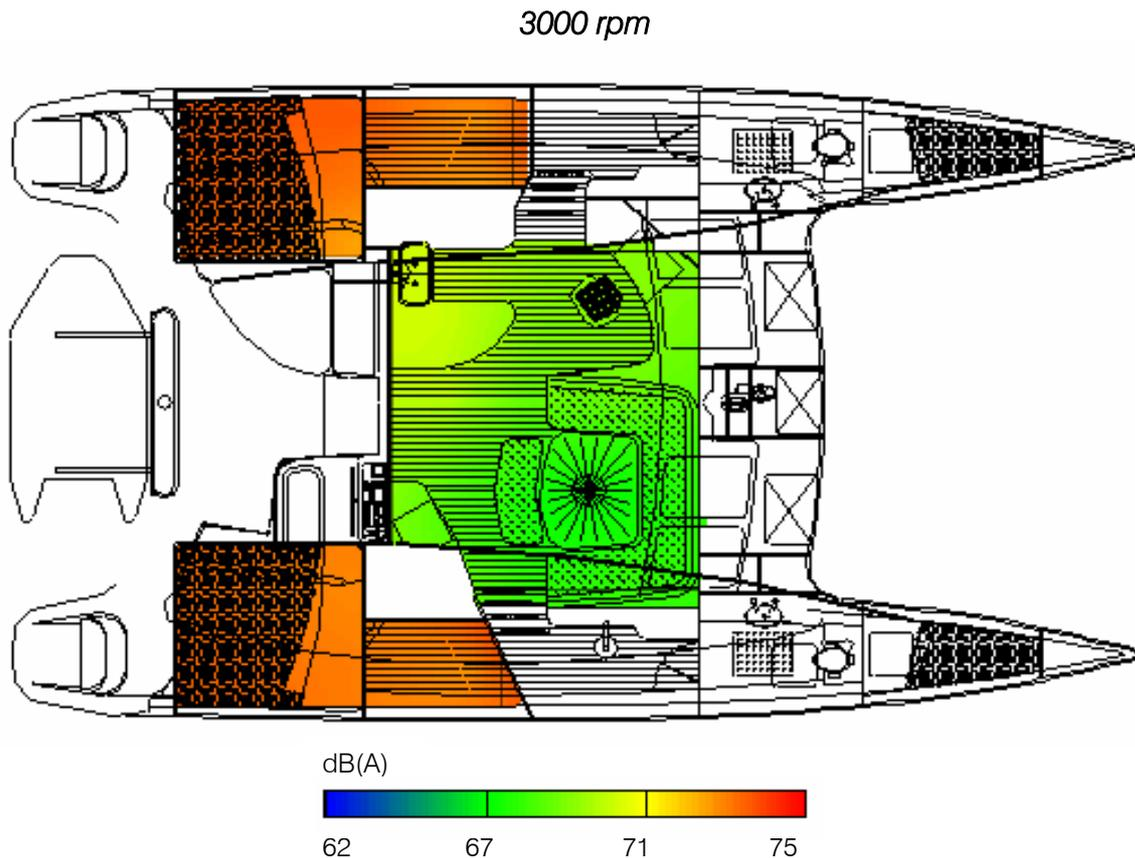
Once again, highest levels are measured for the rear cabins with 74.3dB(A) for the right cabin and 75.2dB(A) for the left. In the main cabin, levels rise from 66.7 to 69.2dB(A)
