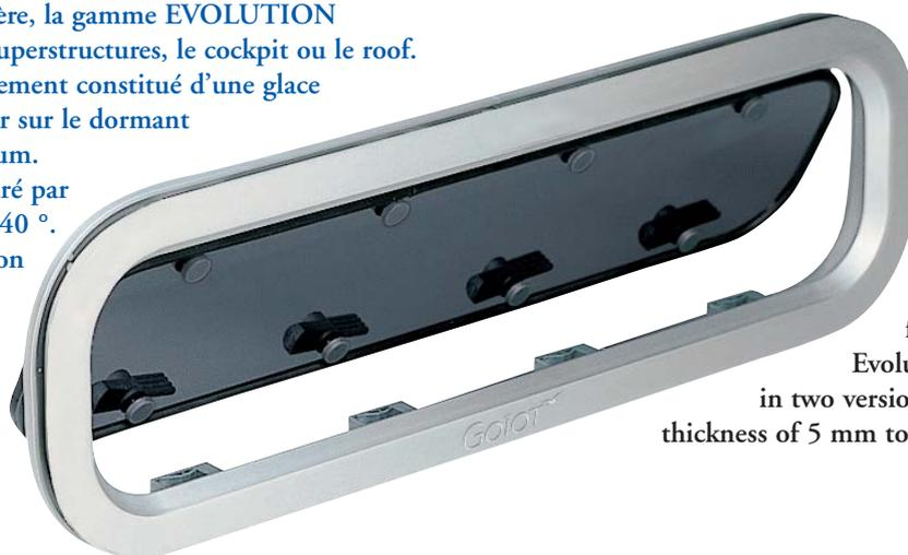
The EVOLUTION ports have a lightweight structure and are ideally suited for the cockpit, the roof or superstructures. The acrylic lid is closing on an extruded profile frame. The 40° angled outside frame is designed to facilitate water draining.
