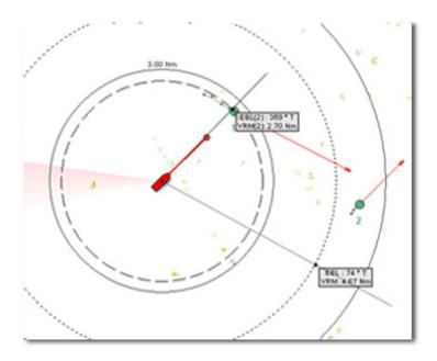
Tool tips are displayed on screen which informed at any time about the EBL (Line representation in the picture) and VRM (ring representation in the picture) range. This can be useful to follow up a point on screen when turning off Radar.
