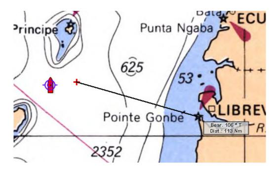
A mark (red cross) is displayed on the chart and recorded in the <u>active layer</u>. The trace line of the bearing remains displayed on the chart.
