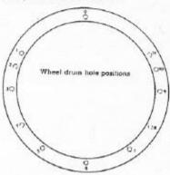
Hole 'O' is marked with a white dot. The following table indicates the holes to be used for differing numbers of wheel spokes.
