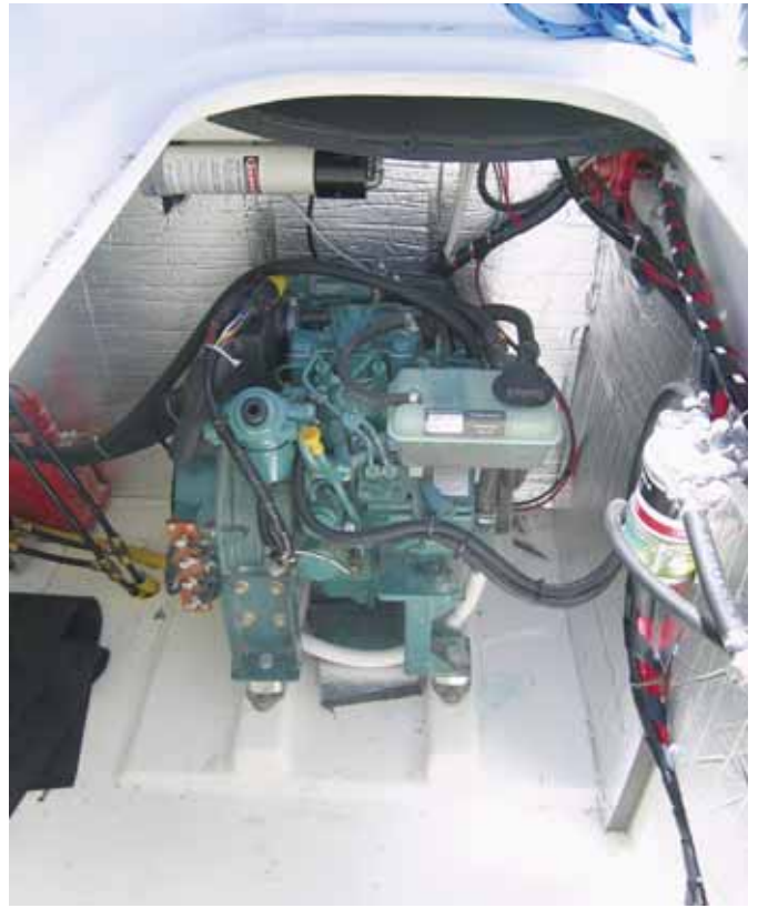
Volvo Penta 12.2hp diesel and 5.4kW 48 volt generator.
