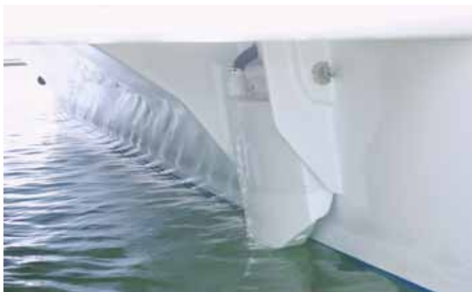
Swing arm in down position. (above left) Torqeedo outboard leg mounted on swing arm – fully up. (above right)
