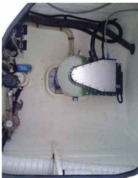
Fusion electric drive 21hp (15.6kVA) electric motor mounted directly on to the saildrive – and a lot of empty space. (left)
