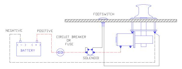
**Step 1:** Make sure the power is on. To test for power use a voltmeter putting the positive probe on the hot, or incoming side of the solenoid, and the negative probe on the ground. See below. If you have 12 volts here then your system is energized and power is flowing though any electrical protection to the solenoid. If you have voltage here proceed to step 2.
