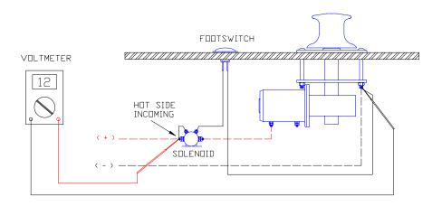
Almost all windlass systems originate at a battery. The cables running from the battery to your windlass are large, as large or larger than your index finger. Follow the positive cable forward to find the electrical protection device. The protection, either a fuse or a circuit breaker is installed breaking the positive cable at some point between the power source and the windlass motor.
