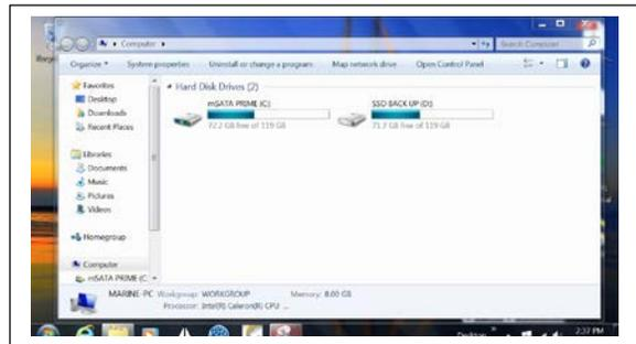
The 1101 Back Up SSD Option is fully prepared before shipment and requires no user action on first install. The Back Up Drive (D:) has the complete image of Drive (C:). The inclusion of this option can be verified with Start>Computer.
